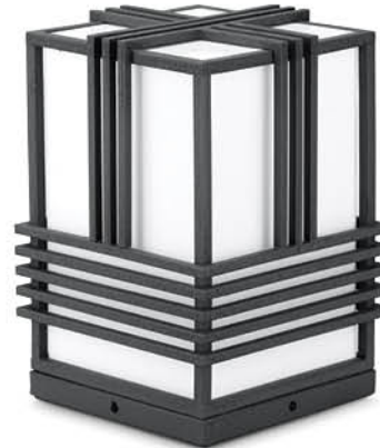
Product Code : 5247 GL Material : MS with MRF Coating + Acrylic Diffuser Finish : Crinkle Grey Dimension : L 260 mm W 260 mm H 395mm Holder: B 22 | IP Rating: IP 54
