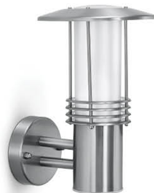
Product Code : 049 WL Material : 304 Grade Stainless Steel+ PC Diffuser Finish : SS Finish Dimension : W 190 mm H 270 mm Holder : E27 | IP Rating : IP 54
